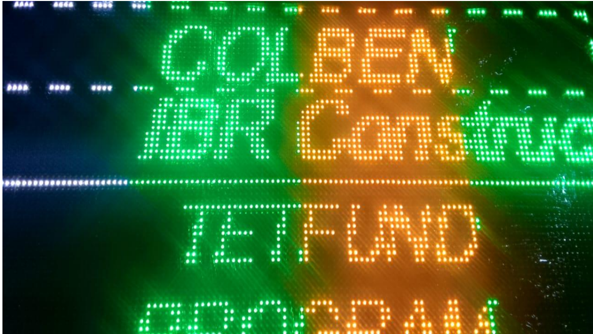
Fig 3. Digital display system with all the P10 module connected in series.
